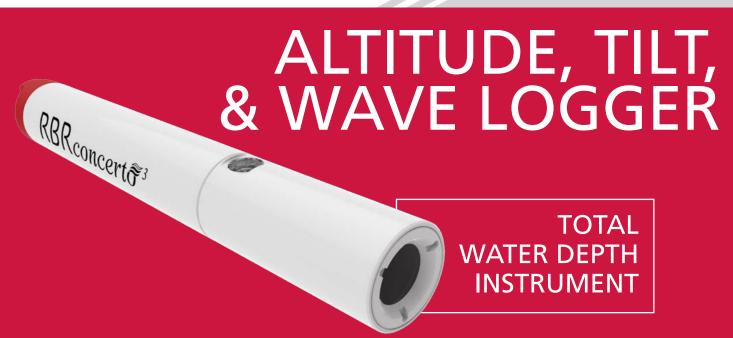
The RBRconcerto<sup>3</sup> D.alt.tilt is a unique data logger dedicated to total water depth. Equipped with a 3-axis tilt sensor and a 200kHz altimeter, the logger provides complete distance-to-surface and distance-to-bottom data. The instrument also includes a depth channel capable of both continuous and intermittent bursts. The RBRconcerto<sup>3</sup> D.alt.tilt is available in a configuration that supports wave measurements up to 16Hz.
